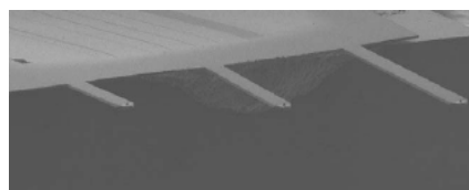
SEM image of the three cantilevers
